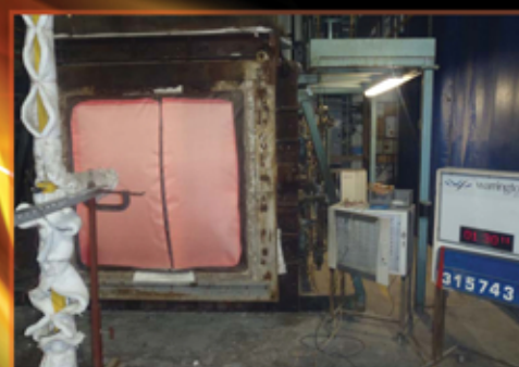
Phoenix after 90 mins on a furnace at 1200° C
